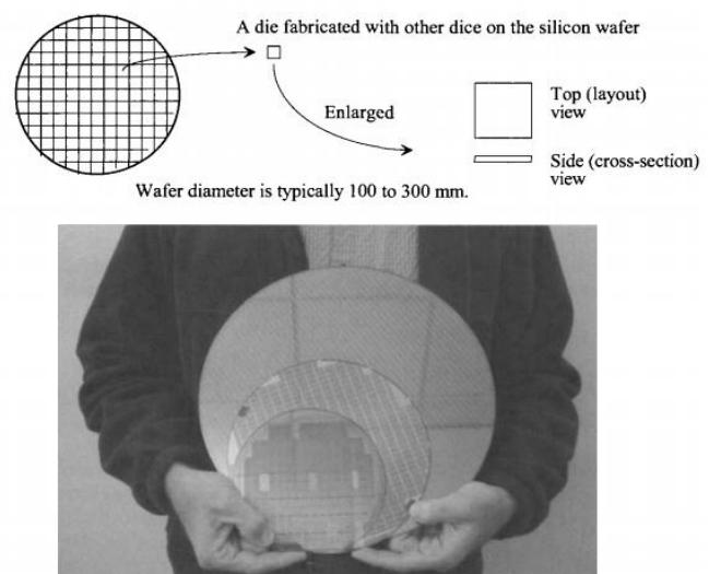
CMOS integrated circuits are fabricated on thin circular slices of silicon called wafers. Each wafer contains several (perhaps hundreds or even thousands) of individual chips or "die".
